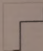
Outside (or 270°) L, right-handed, plan ("Outside," because the view is "outside" the angle enclosed by the L.)
